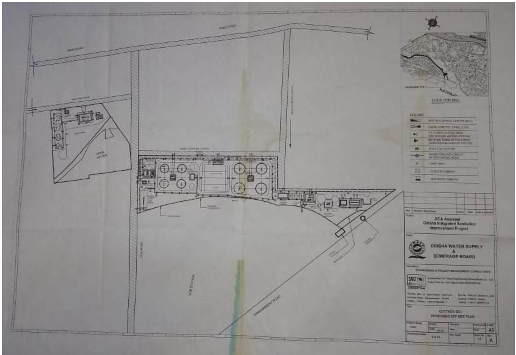
Fig. 15 Schematic diagram of STP to be constructed in Sewerage District-I of Cuttack city
